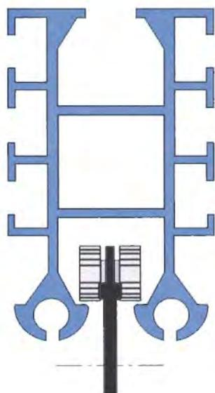
The 2-way Combi-Rail can be used universally. It is used to hold stage curtain rolls, trolleys and heavy duty castors.
