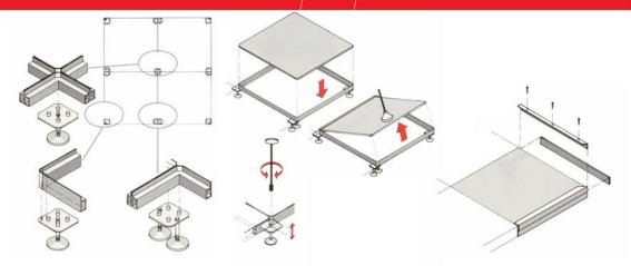
Alu-Plano exhibition floor system is extremely easy to assemble and dismantle. The feet for the central, edge and corner areas can also be adjusted after the floor has been set up. The adjusting screw is covered with a suitable plug. As a conclusion, the entire area is surrounded by a panel, which consists of angled and flat profile.
